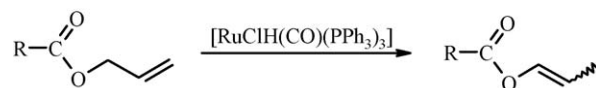
Scheme 10. Isomerisation of allyl carboxylates catalysed by [\text{RuClH}(\text{CO})(\text{PPh}_3)_3] [21,37,50]. (a) R = Me, Bu; y = 45\% ( E/Z = 0.3 ); t = 60^\circ\text{C} ; \tau = 3 h; 10 mol% [Ru]. (b) R = MeO; y = 80\% ( E/Z = 0.4 ); t = 80^\circ\text{C} ; \tau = 6 h; 13 mol% [Ru]. (c) R = Ph; y = 80\% ( E/Z = 0.4 ); t = 120^\circ\text{C} ; \tau = 3 h; 10 mol% [Ru].
